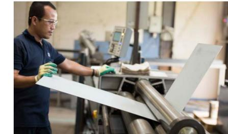
Pressbreaks can fold up to 3m long, max 15 mm thick for steel. CNC rolling from radius 60-1500 mm, max thickness 4 mm for steel.
