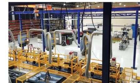
High pressure cabinet leak test stations with overhead gantries.
