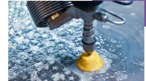
Waterjet Cutting machine capabilities up to 100 mm for steel, Stainless, Aluminium and Polycarbonate material.
